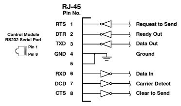
Figure A.1: Serial Port Interface
